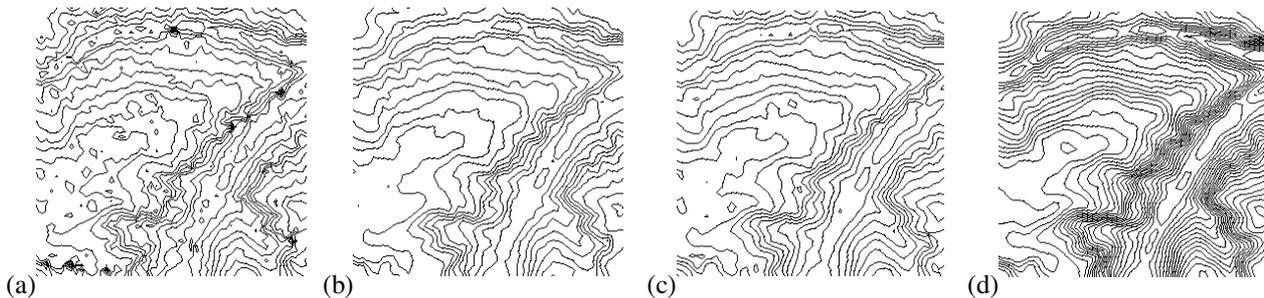
Figure 4. DTM filtering and smoothing. (a) Original DTM with many outliers; (b) Rank-based filtering, 5 iterations; (c) Bicubic -  $\sigma$ -filtering,  $\alpha=1$ ; (d) Spline smoothing, 5 iterations
