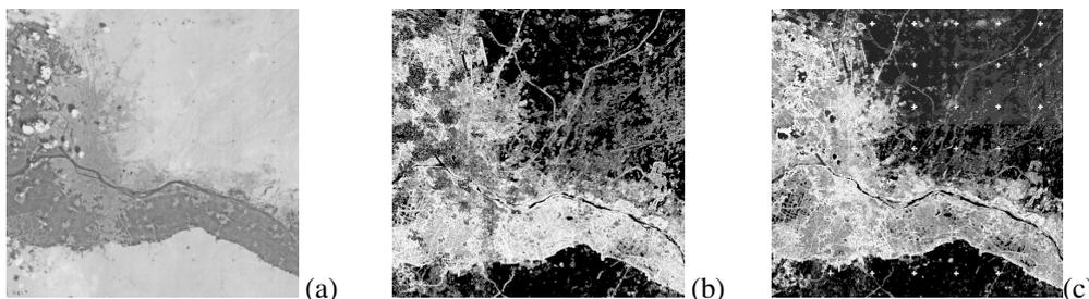
Figure 1. A priori and a posteriori evaluations of signal level inside templates. (a) Original image (left image of the stereopair). (b) Correlation coefficient as a posteriori evaluation of a signal level inside templates (the coefficient values from [0,1] are transformed to the gray-level range [0,255]). (c) A variance of a template brightness as a priori evaluation of a signal level inside templates (variance values are transformed to the gray-level range [0,255]).
