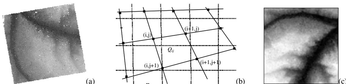
Figure 3. Regular DTM matrix creation. (a) Regular matrix of horizontal disparities (values are transformed into the brightness range 0..255). (b) This figure schematically shows a disposition of matched points projected in object space. The dashed lines show a regular DTM matrix that should be obtained from known 3D-points. The coordinate axes are oriented along geodesic axes. (c) Result of the regular DTM matrix creation (height values are transformed to the brightness range 0..255).
