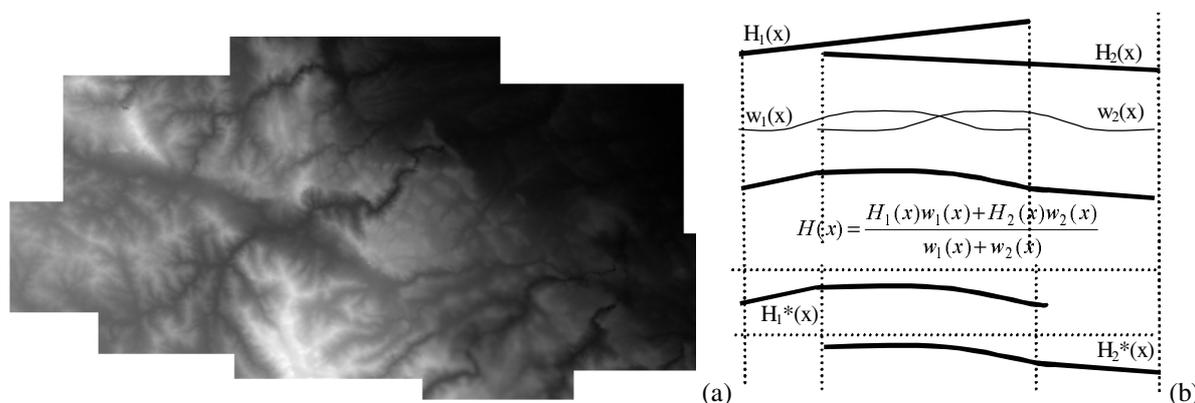
Figure 9. DTM merging. (a) Result of eight overlapped matrices with a resolution 10m merging. The resulting DTM cover region 90km by 50km with a resolution 10m. (b) Illustration of the algorithm. The profiles of two overlapped DTMs  $H_1, H_2$ , appropriate weighting functions  $w_1, w_2$ , and the result of merging  $H$  are shown. Also the results of original DTM correction  $H_1^*, H_2^*$  are shown.
