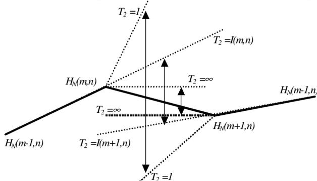
Figure 7. Evaluation of an altitude range on an interval  $(m,n)-(m+1,n)$  with the help of geomorphologic index. The thick line shows a DTM profile. The dashed lines show values  $H^*_{mn}$  and  $H^*_{m+1,n}$ , obtained from (10). As examples three values of the parameter  $T_2$  are taken. The arrows show appropriate evaluations of an altitude range obtained from (9).
