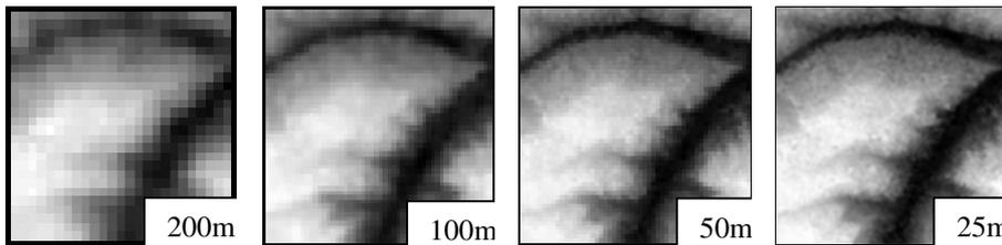
Figure 6. Hierarchical scheme of DTM generation. The DTM pyramid and resolutions at appropriate levels are shown.
