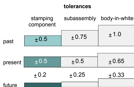
Figure 1: Development of the tolerances in the automotive industry
