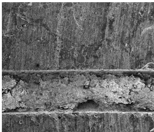
Figure 10. SEM image of sample after friction process (25:1)
