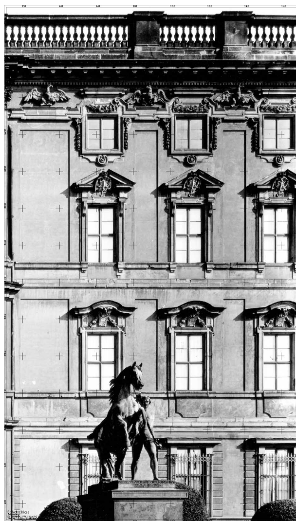
Figure 5: A Meydenbauer image of the “Stadtschloss”, rectified to control points as determined by a bundle block adjustment, superimposed by a 2m grid.
