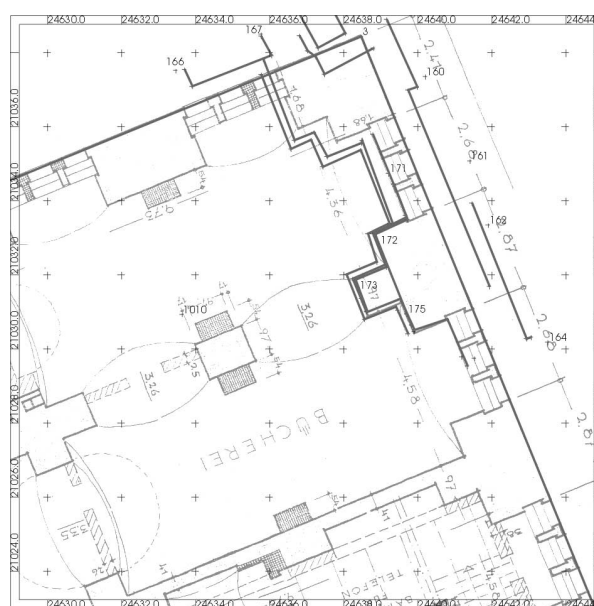
Figure 3: A historical basement plan of the Bauakademie rectified to the calculated building corners and superimposed by the survey of the excavated fundaments.
