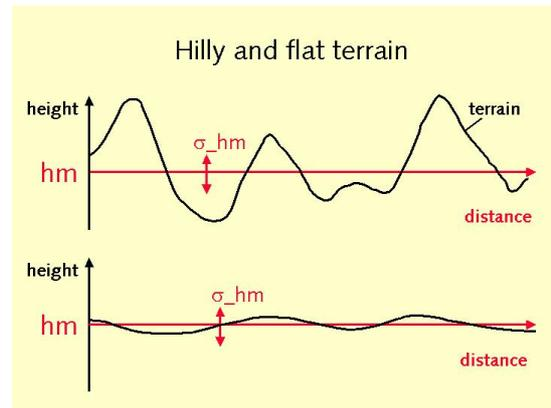
Figure 3. The precision of the mean field height (hm) is *not* dependent from the terrain type.
