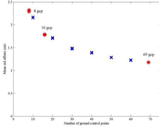
Figure 11. Mean standard deviations of all strips (except cross strips) for different numbers of ground control points.
