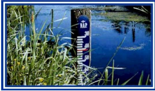
Figure 2. Water-gauge for measuring water levels.
