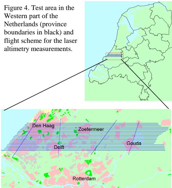
Figure 4. Test area in the Western part of the Netherlands (province boundaries in black) and flight scheme for the laser altimetry measurements.
