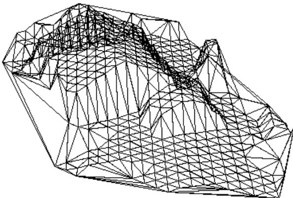
Figure 2-1. A building's point cloud with TIN-structure
