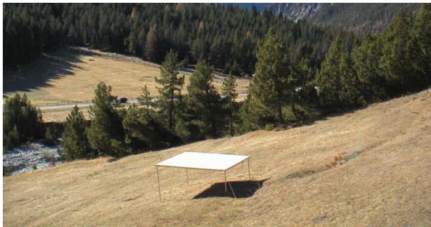
Figure 2: View of the Ofenpass area with two (one in the upper corner of the background meadow) geometric reference targets. The top of the targets was constructed using cardboard.
