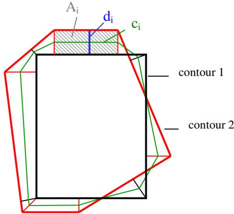
Figure 14. Area based approach for positioning accuracy analysis
