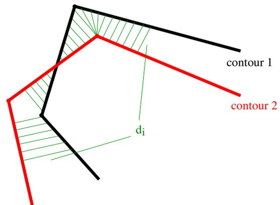
Figure 13. Discretisation approach by pointwise determination of shortest distances  $d_i$
