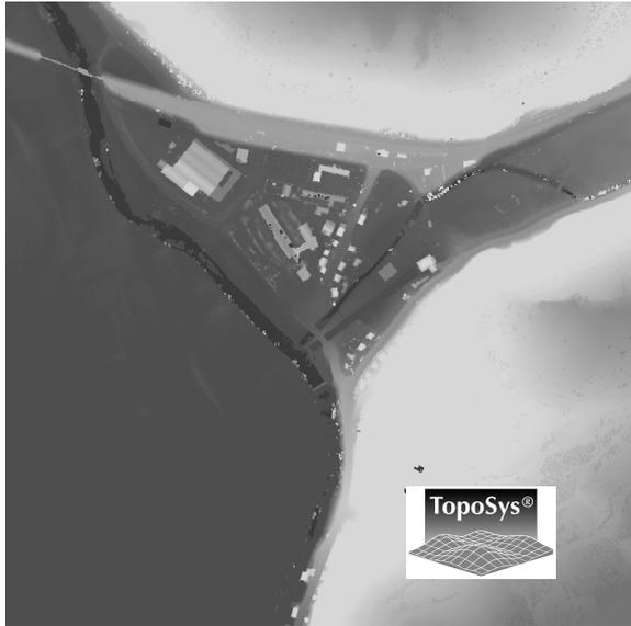
Figure 1. Original laserscanning raster data (DSM), pixel size 1m, test area 'Fridingen' (1 km x 1 km)
