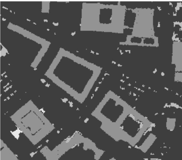
Figure 10. Classification result for test area 'Karlsruhe' (dark grey: buildings, light grey: trees, white: terrain objects)
