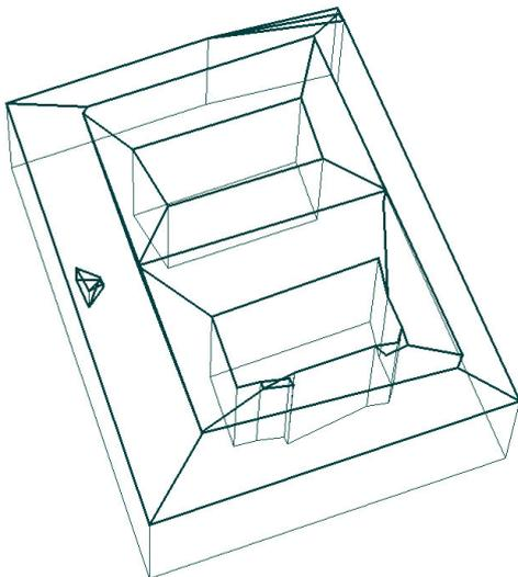
Figure 12. Extracted building edges and corner points by intersection of vertical and roof planes
