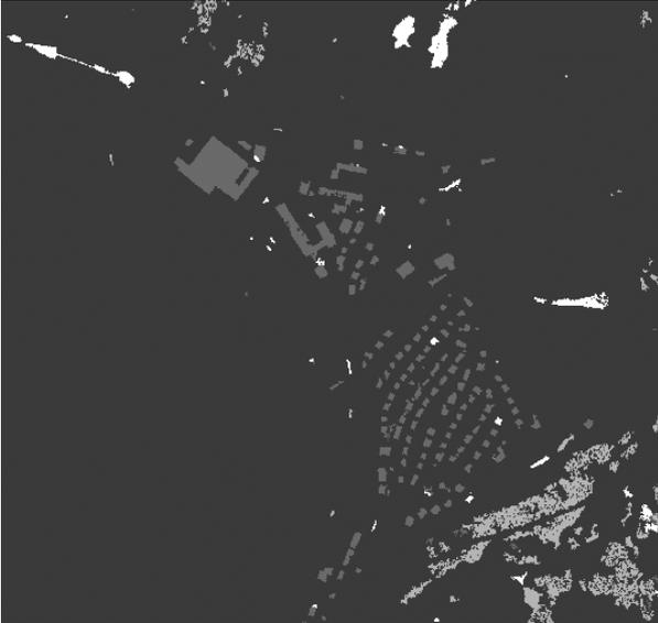
Figure 9. Classification result for test area 'Fridingen' (dark grey: buildings, light grey: trees, white: terrain objects)
