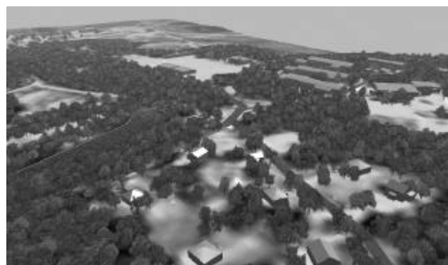
Figure 7. A high-resolution digital terrain model including trees and buildings. Besides the textures all parts of the model are derived from laser scanner data.
