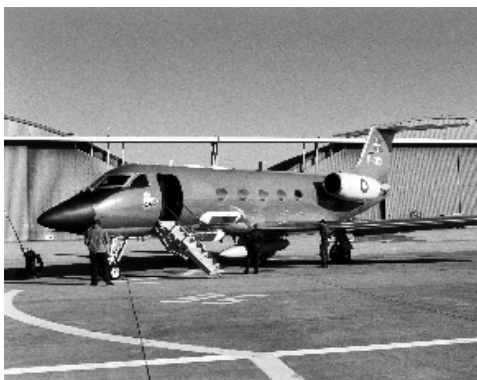
Fig. 5. G3 with EMISAR XTI radar
