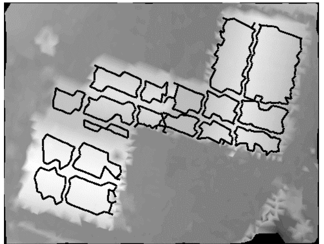
Figure 3: Bounds of planar faces detected by the 3D Hough transform within the partitions.
