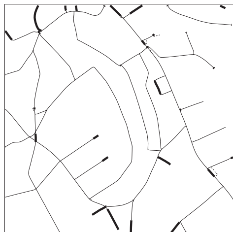
Figure 5: Extraction using network properties (thin lines: correct extraction; thick lines: missing extraction; dashed lines: incorrect extraction)
