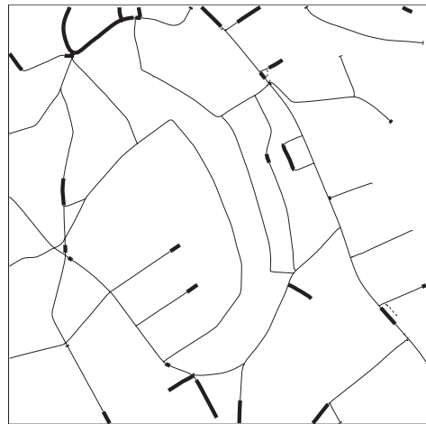
Figure 4: Extraction using local grouping (thin lines: correct extraction; thick lines: missing extraction; dashed lines: incorrect extraction)
