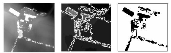
Figure 2. Given DSM (250 m • 250 m; left), results of segmentation (middle) and classification (extracted regions that have to be reduced are in black; right)
