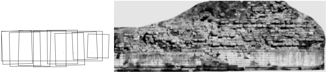
Figure 1: Project “Sparta”: footprints of the image strip and corresponding part of the final orthoimage
