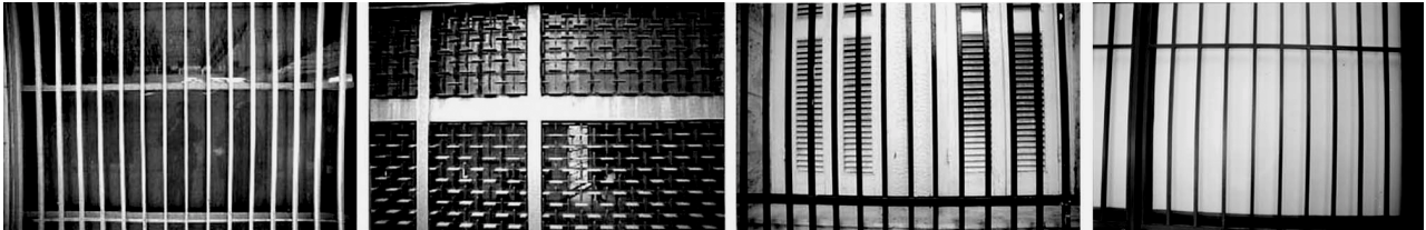
Figure 5: Small-format images from different lenses (three with f = 17 mm, one with f = 24 mm) used for estimation of distortion
