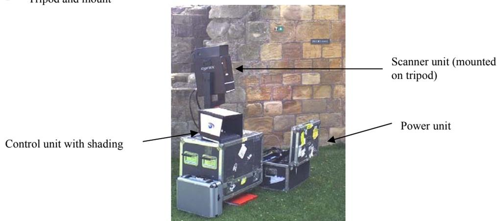
Figure 3: An example scanner system - Cyrax 2400
