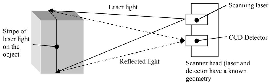
Figure 1: A triangulation system. The laser stripe is sampled along its length.
