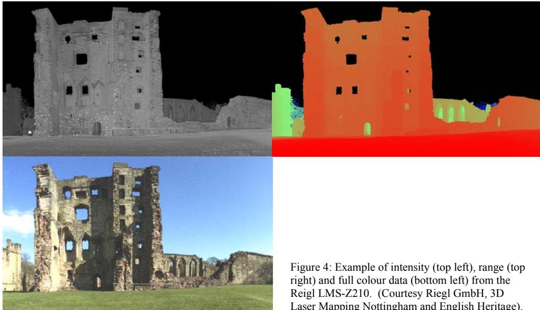
Figure 4: Example of intensity (top left), range (top right) and full colour data (bottom left) from the Riegl LMS-Z210. (Courtesy Riegl GmbH, 3D Laser Mapping Nottingham and English Heritage).
