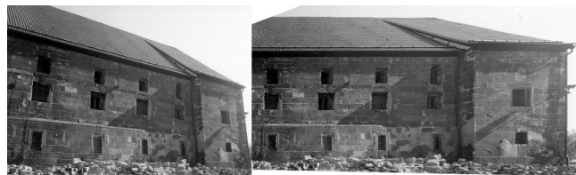
Fig. 5: Image rectified by one known window aspect ratio
