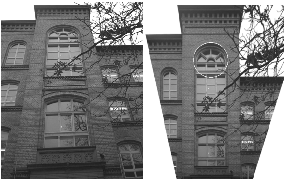
Fig. 4: Original image and rectified plane using a circle arc
