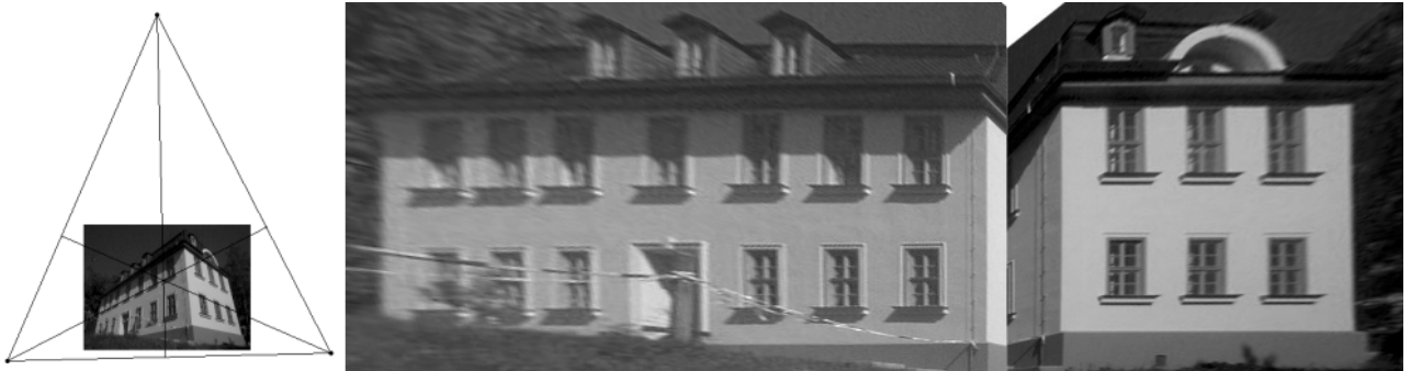
Fig. 3: Original image with vanishing point triangle and principal point, rectified facades
