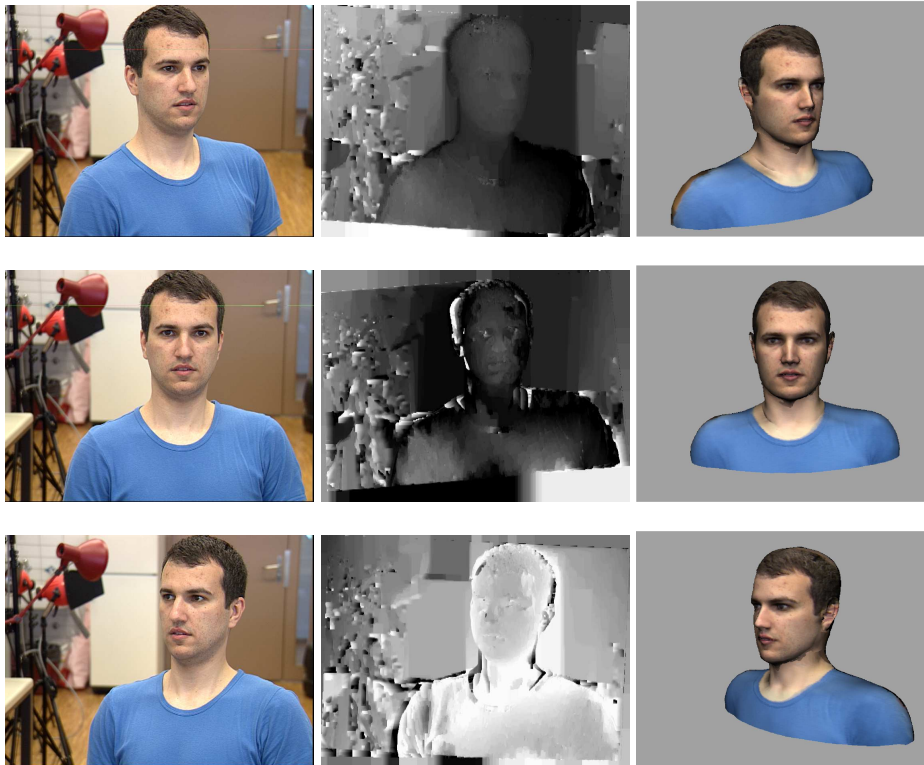
Figure 1: Reconstruction from an uncalibrated video sequence. Left column: 3 of 6 images from a short video sequence. Middle column: Disparity maps extracted from consecutive image pairs using correlation-based stereo. Right column: Reconstructed and textured models obtained by using an explicit model for the head and an implicit mesh model for the neck and shoulders.
