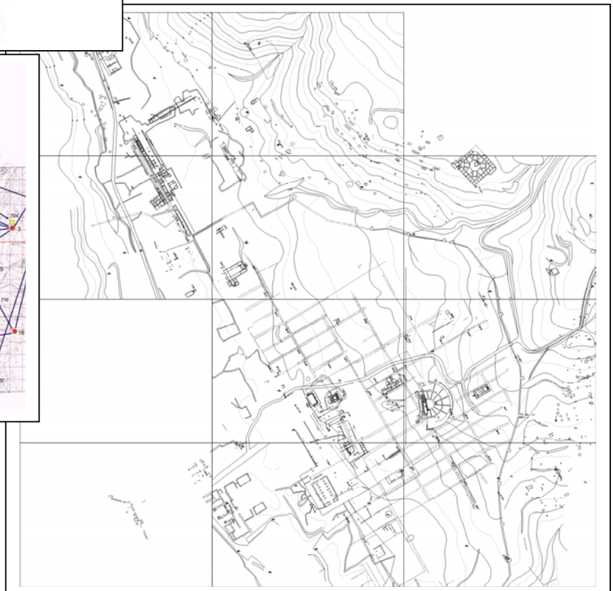
Figure 3 – Topographic intersections on searched out points; they are purposed to compute a rubber sheeting registration of two datasets.
