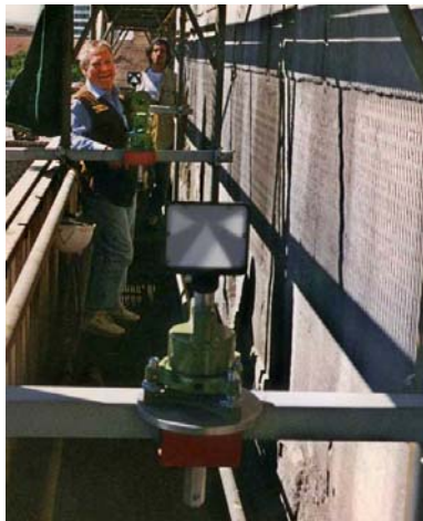
Figure 3. During the surveying operations. The theodolite and the targets are visible
