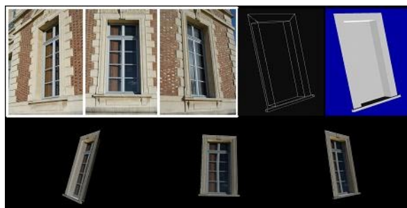
Figure 6. Example of the downstairs window. The 3 initial images are on the top-left. On the top-right, there are the wire-frame and the surface model. On the bottom, the final model of the windows with accurate texture.
