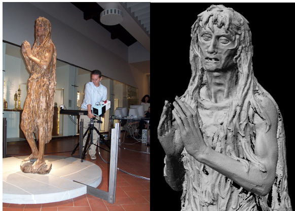
Figure 13 – 3D scanning: a) relocation of the 3D scanning system around the statue; b) 3D model (F.Costantino, G.Guidi, D.Ostuni)
