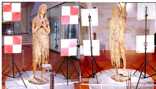
Figure 15 - Photogrammetry setup: measurement targets nearby the manufacture: a) front view; b) rear view
