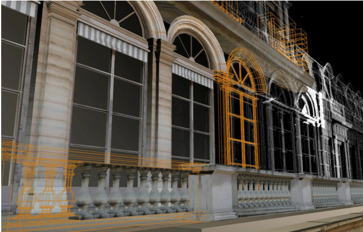
Fig 11. Result of the modeling showing the point cloud, the textured and the wireframe model.
