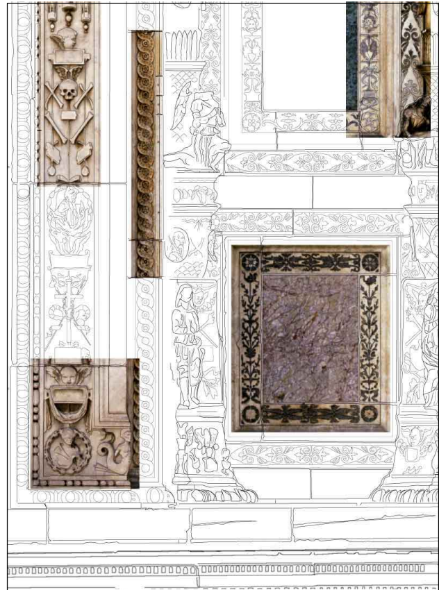
Figure 11. The window of the “right-hand fifth”: orthogonal projection of the restitution model (original on a scale of 1:10)
