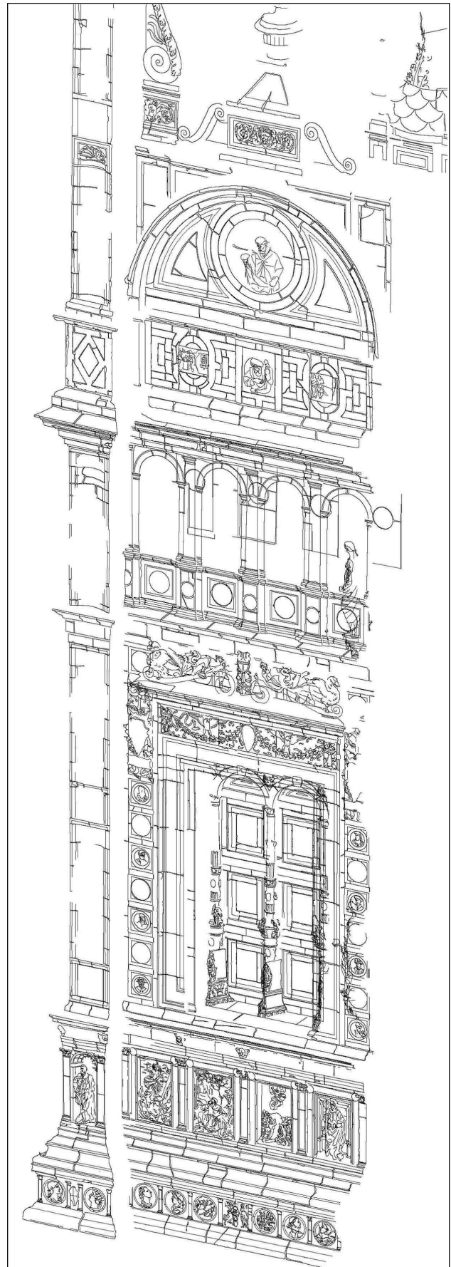
Figure 8. The “right-hand fifth” of the façade: axonometric projection of the restitution model (original on a scale of 1:50)
