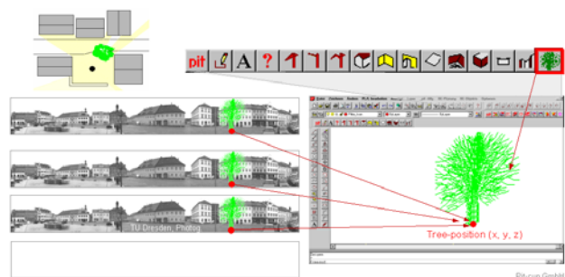
Figure 11. Photogrammetry functions should replace the pointer of mouse in CAD systems (Source: TU Dresden, Pit Cup GmbH).
