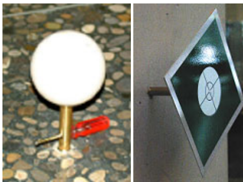
Fig. 6: Sphere (left) and target (right) with used adapter
