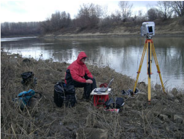
Fig. 14: Scanner and equipment in use at the river Tisza
