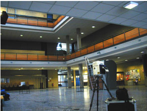
Fig. 5: GS100 in the 3D test field of HAW Hamburg
