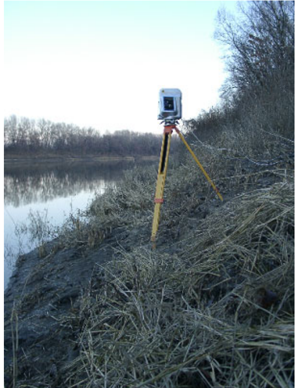
Fig. 15: Scanner in a warped embankment of the river Tisza
