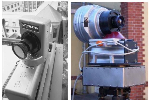
Fig. 26: Digital panorama line-scanning cameras RotaScan Noblex (left) and KST EyeScan M3 (right)
