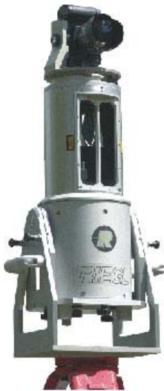
Fig. 28: 3-D laser-scanner with integrated camera (Riegl)
