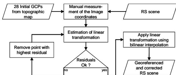
Figure 11. Workflow of the georeferencing procedure
