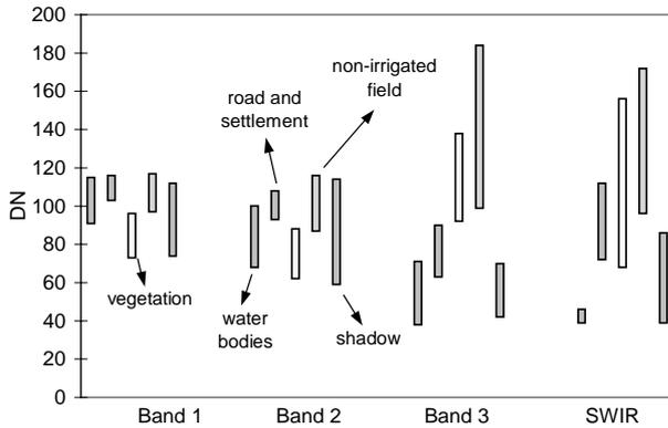
Figure 5. The spectral response range for typical object classes in SPOT2 XS resp. SPOT4 XI multispectral data
