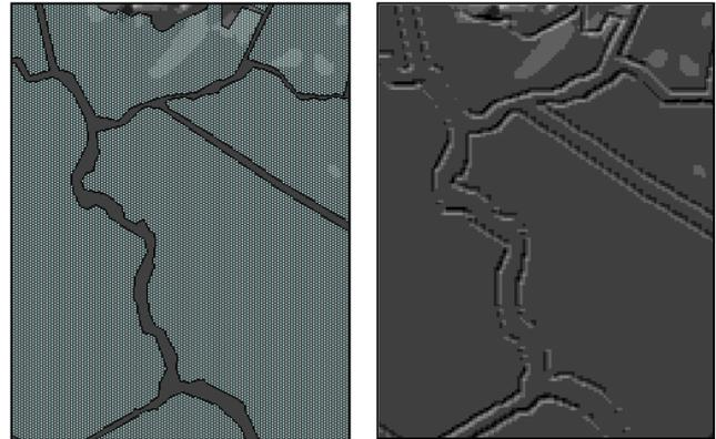
Shaded 50 m DEM with polder areas      50 m DEM with 2 m walls at polder boundaries
