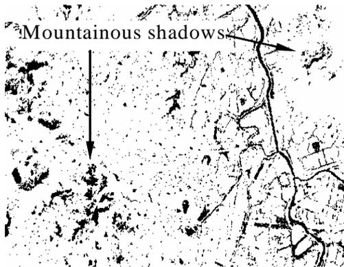
Figure 6. Water image extracted using thresholding at SWIR
