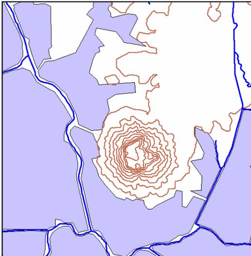
Figure 3. Input data for the DEM generation: Elevation zones (contour lines), oriented river middle axis, water bodies and polder areas
