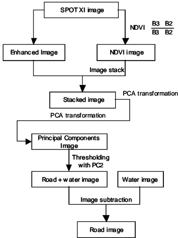
Figure 8. The procedure of road extraction
