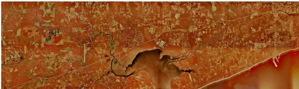
Figure 3. The Computational Mapping Engine was used to mosaic twenty quads of digital ortho-imagery and transform the resultant image to a custom map projection. These images exceed 50MB per file in raw format, requiring extensive storage. Creating custom products from such image files requires numerous complex steps and is a time consuming process if done using tradition methods.
