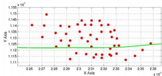
Figure 4. Aircraft trajectory and GCPs distribution in local tangent system.
