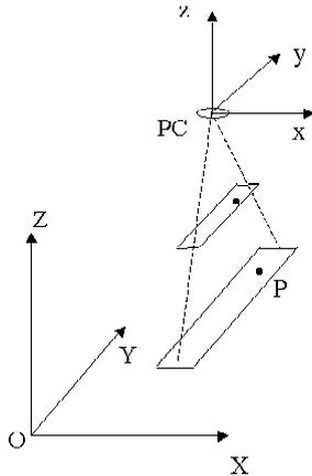
Figure 1. Image coordinate system with origin in instantaneous perspective centre (PC) and ground coordinate system with origin in O.
