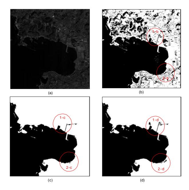
**Figure 1** Experiment results for coastal line feature extraction. (a) Source remote sensed image, (b) Binary image after processed by gray threshold approach, (c) Coastal line feature extracted by conventional threshold approach, (d) Coastal line feature extracted by proposed approach.
