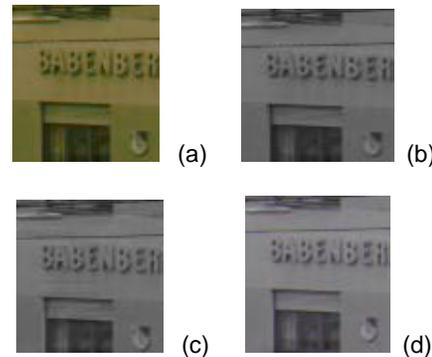
**Figure 4:** Example of a color image using the Bayer-pattern. (a) Color. (b) Green channel 1 @ mean gray value 106; (c) Green channel 2 @ mean gray value 111; (d) False color using the three channels green1, green2, 0.5\*(green1 + green2).
