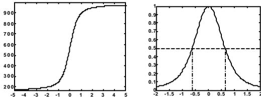
**Figure 2:** The 2D version of the 3D edge function is shown to the left, and is obtained from Fig. 1 (right). The first derivative of this real edge function creates a line spread function LSF. The width of the LSF at 50% of the amplitude is a measure of the geometric resolution (from Blonski, 2002). The horizontal dimensions are in pixels.
