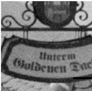
Figure 7: Rollei 6006 image using Ilford FP4 film scanned at 5µm pixels. Taken at 1:1.000 with a 50mm lens from a distance of 50 m. Each pixel is 7mm in object space.
