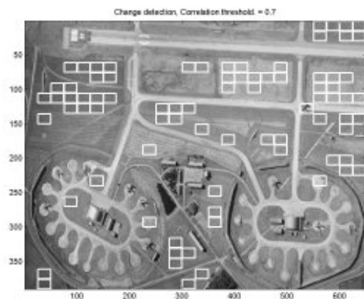
Figure 10 : Image 2 after detection of changes by correlation
