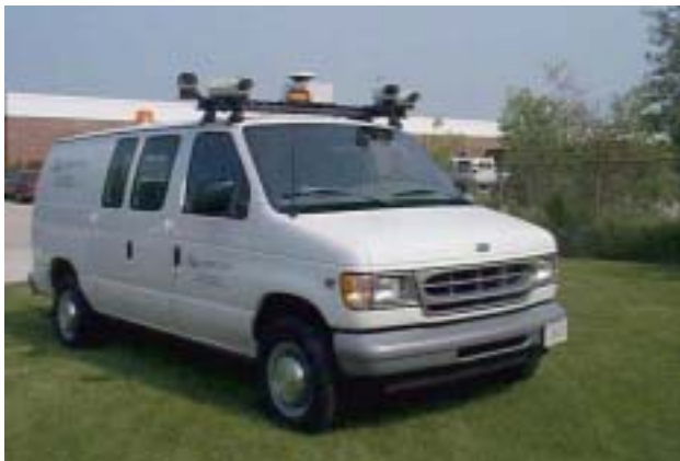
Figure 1. Portable GPSVision system consists of GPS, INS and four digital cameras
