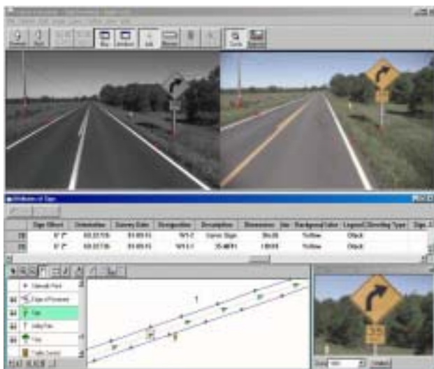
Figure 3. Stereo images are used to locate and measure roadway infrastructure.
