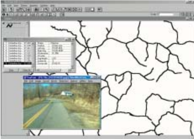
Figure 5. Road centerline with attributes and links to the digital images
