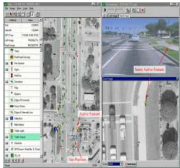
Figure 7. The GPSVision data overlaid on the aerial photography. This provides the view of the infrastructure both from the ground and in the air. It is used for engineering design.
