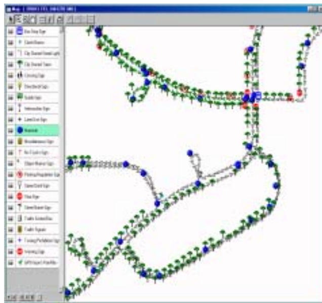
Figure 4. Roadway assets, like traffic signs, poles, guardrails, etc. are extracted from the GPSVision mobile mapping system
