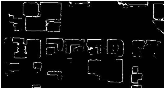
Figure 4 Result after applying Sobel on airborne laser data
