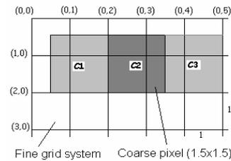
Fig. 1 - Coarse data mapped on the enhancement grid
