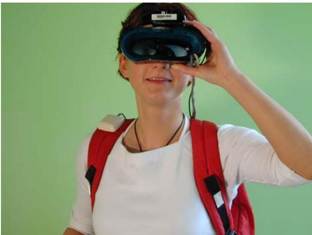
Figure 1: Hand-held display with orientation tracker
