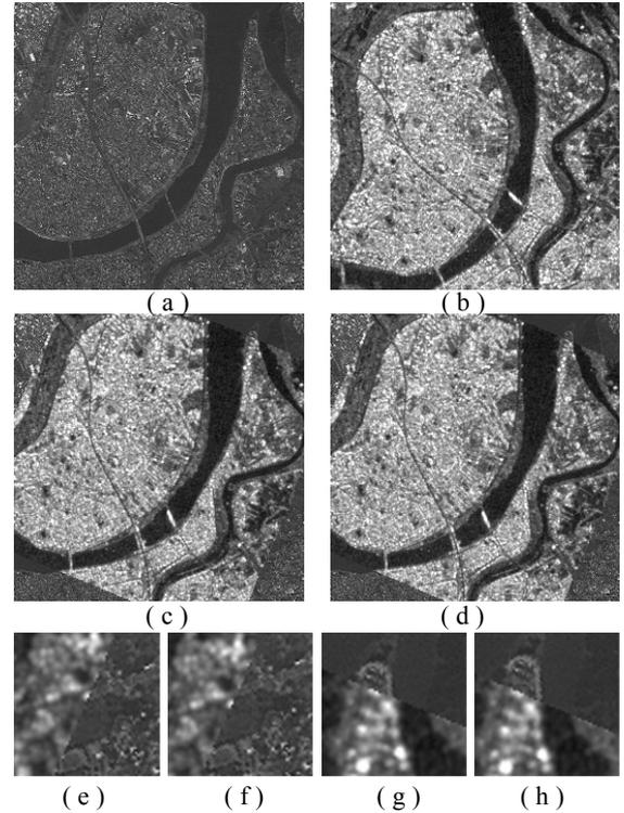
Fig. 3. (a) SPOT image; (b) SAR image; (c) registration by manual; (d) registration by our method; (e) and (g) are two sub images cut from the image shown in (c); (f) and (h) are two sub images cut from the image shown in (d).
