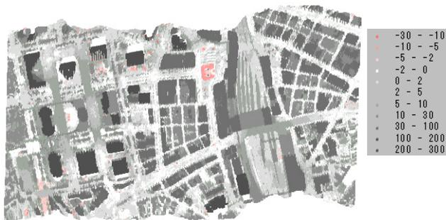
Figure 3. Difference of DSM and approximate DTM
