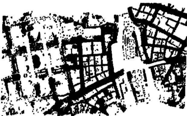
Figure 4. Laser-observed points whose height difference from the approximate DTM is within  $\pm 1$  m
