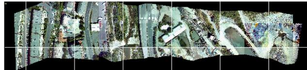
Figure 9: Orthophoto generated from laser DSM and digital photo.
