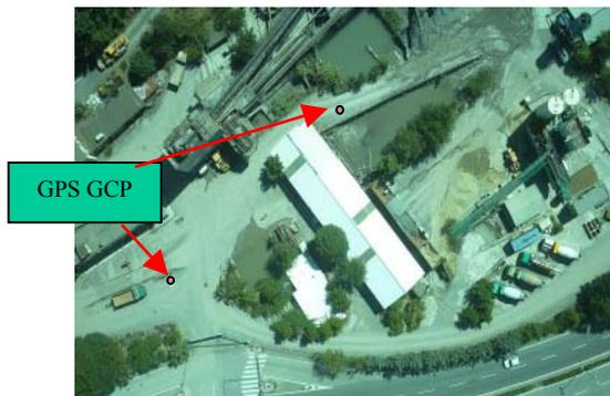
Figure 4: Location of Two GPS ground control points.
