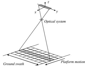
Figure 2 – Image acquisition by a linear array scanner
