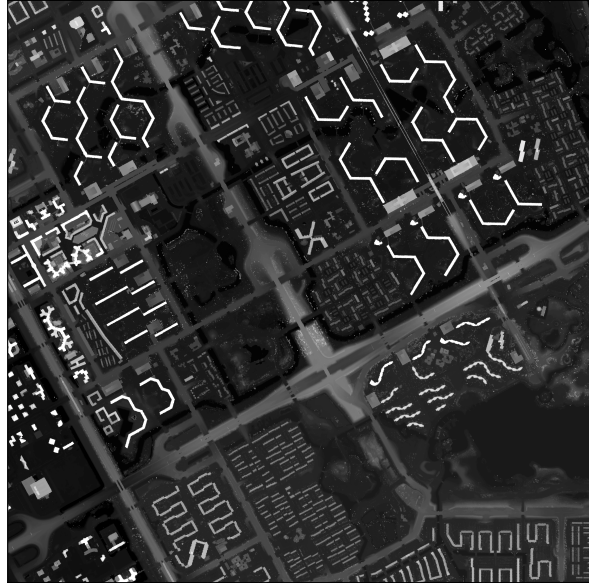
Figure 6. Laser scanning data (AHN) with 1 m resolution (Copyright hold by Rijkwaterstaat, the Netherlands)
