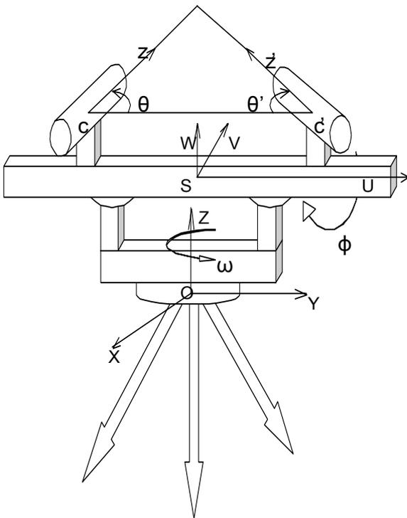
Fig.1 A basic physical structure of Photogrammetron-I
