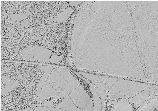
(a) Interpolated original LIDAR data
