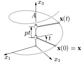
Figure 1: Helical motion.
