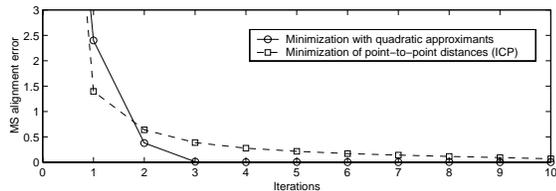
Figure 4: Comparison of the convergence rate for our method vs. minimization of point-to-point distances in each step (ICP).
