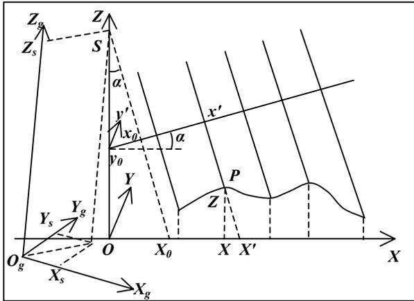
Fig.1 Imaging Geometry of Parallel Ray Projection
