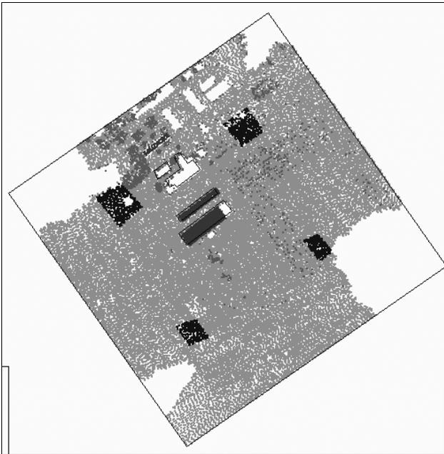
Figure 5. System calibration flight 2, four strips flown for misalignment calibration. Dark areas (flat surface and roof structures) were used for matching.
