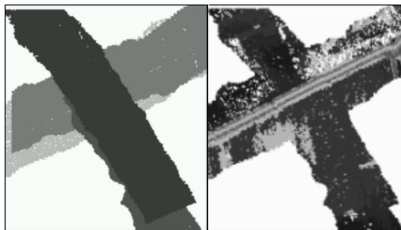
Figure 3. System calibration flight 1, four strips flown for misalignment calibration. Left: strips. Right: elevation.
