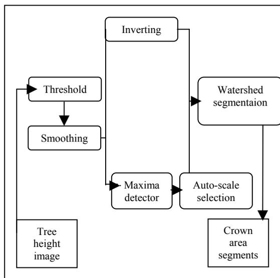
Figure 4: Working steps for single tree segmentation
