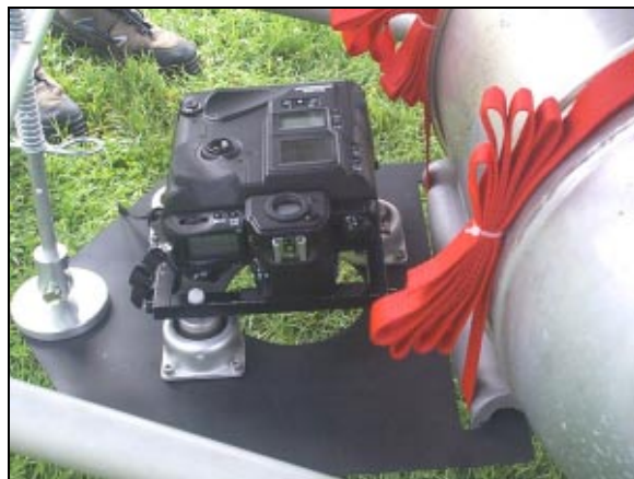
Figure 7. Kodak DCS 660 digital camera mounted in the Thruster microlight
