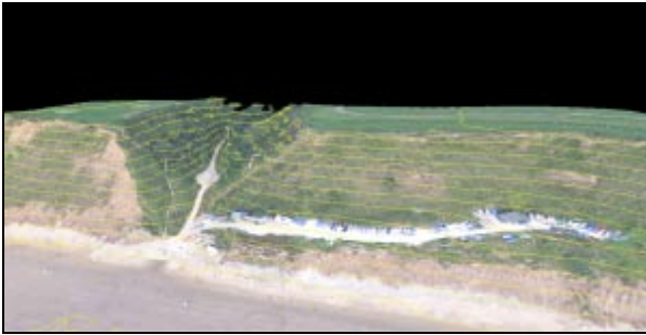
Figure 9. DEM generated in LH Systems SOcET Set from the Kodak DCS 660 aerial imagery (3 m contours)
