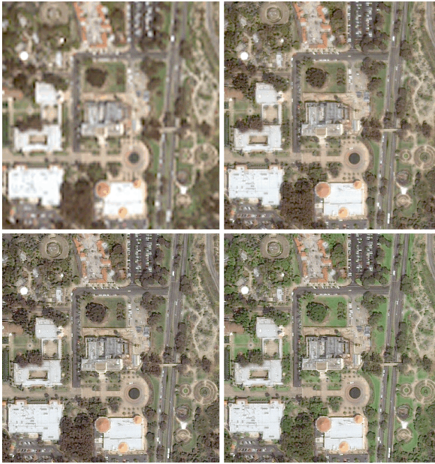
Figure 9. Effects of three fusion models of the new fusion technique. (a) Original IKONOS 4 m natural colour image, (b) Fusion result of the spectra preserving model. (c) Fusion result of the spatial detail preserving model. (d) Fusion result of the colour enhancing model. (with a: upper left, b: upper right, c: lower left, d: lower right)
