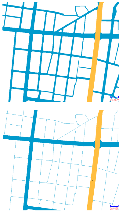
Figure 7. Simplified result. Upper image: original roads (1/2500), lower image: simplified results (1/25000)
